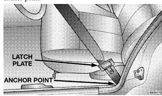
2. At about 6 to 12 inches above the latch plate, grasp and twist the belt webbing 180° to create a fold that begins immediately above the latch plate.
