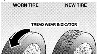
These indicators are molded into the bottom of the tread grooves and will appear as bands when the tread depth becomes 1/16 inch (2 mm). When the indicators appear in 2 or more adjacent grooves, the tire should be replaced.
