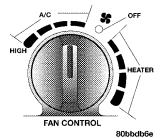
Use this control to regulate the amount of air forced through the system in any mode you select. The fan speeds to the left of the OFF position are for Air Conditioning. Choosing one of these speeds turns on the air conditioning compressor. The fan speed increases as you move the control counterclockwise from the OFF position.
