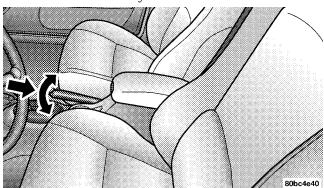
When parking on a hill, it is important to set the parking brake before placing the gear selector in Park, otherwise the load on the transmission locking mechanism may make it difficult to move the selector out of Park. As an added precaution, turn the front wheels toward the curb on a downhill grade and away from the curb on a uphill grade.
