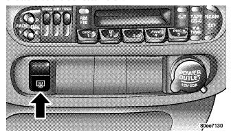
NOTE: The defroster turns off automatically after 10 minutes of operation. Each following activation of the defroster will last for five minutes.
