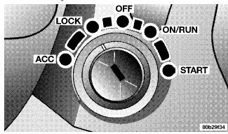
**NOTE:** If you try to remove the key before you place the lever in PARK, the key may become trapped temporarily in the key cylinder. If this occurs, rotate the key clockwise slightly, then remove the key as described. If a malfunction occurs, the system will trap the key in the ignition cylinder to warn you that this safety feature is inoperable. The engine can be started and stopped but the key cannot be removed until you obtain service.
