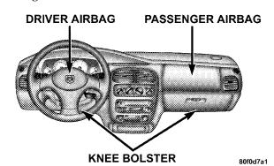
**NOTE:** The front airbags are certified to the Federal regulations that allow less forceful deployment.
