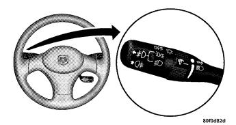
To change the brightness of the instrument panel lights, rotate the center portion of the Multi-Function Control Lever up or down.
