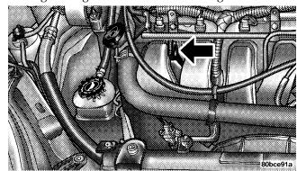
Checking the oil while the vehicle is on level ground will improve the accuracy of the oil level readings. Maintain
