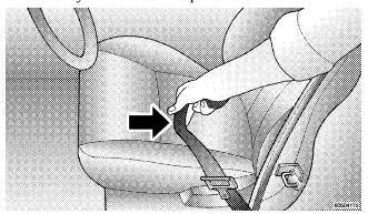
3. Slide the latch plate upward over the folded webbing. The folded webbing must enter the slot at the top of the latch plate.
