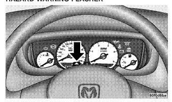
The flasher switch is on top of the steering column, just behind the steering wheel. Depress the switch and both cluster indicators and all front and rear directional signals will flash. Depress the switch again to turn Hazard Warning Flashers off.
