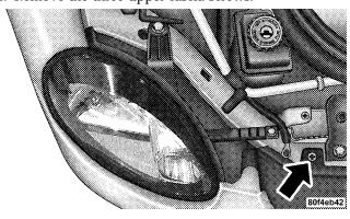
2. Remove two screws from the headlight assembly and remove the assembly from the vehicle.
