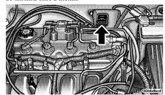
When additional coolant is needed to maintain the proper level, it should be added to the coolant bottle. Do not overfill.
