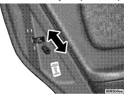
To provide a safer environment for children riding in the rear seat, the rear doors of your vehicle have the child-protection door lock system.
